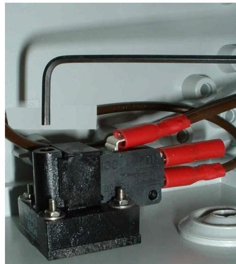
5. Each full turn of the adjusting screw increases/decreases the pressure by ~1 psi (~0.1 Bar).
